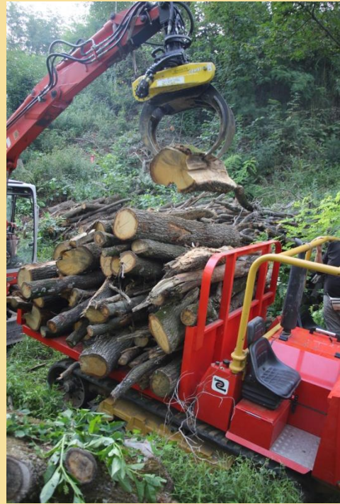
Speed-Track employed in a forest to forward wood.
