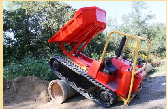
Speed-Track can easily overcome really high obstacles (the diameter of the pipe in the picture is more than 600 mm)
