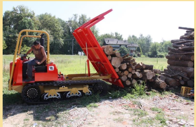
Speed-Track in the configuration with the foldable floor, discharging the load.
